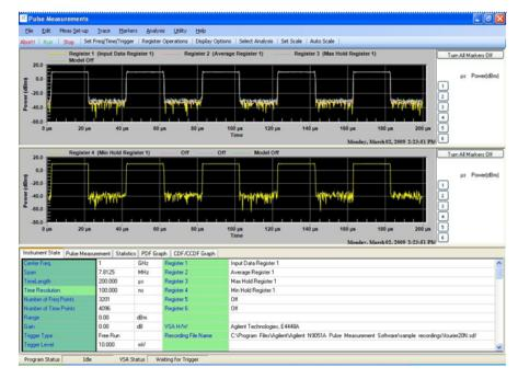
Dual display with average and max hold on upper and min hold in lower display.
